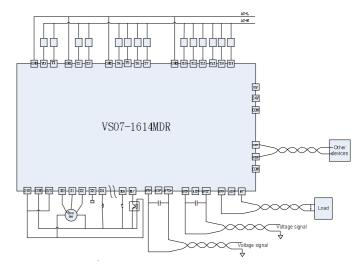
Input connection instance of analog signal
