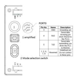
As a specialized interface for user programming, PORT0 can be forcibly switched to the programming port protocol through the mode selection switch. The following table describes the mapping between PLC running states and PORT0 running protocols.
