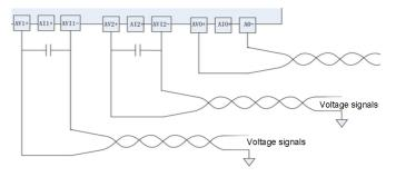
1. For analog input, it is recommended to use shielded twisted-pair cables. The cable should be kept away from the power wire or other wires that may cause electrical interference.
